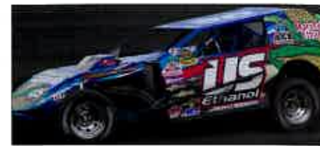
The US Ethanol race car roars around dirt tracks at 90 miles an hour using E98 ethanol in its 350-horsepower engine.
